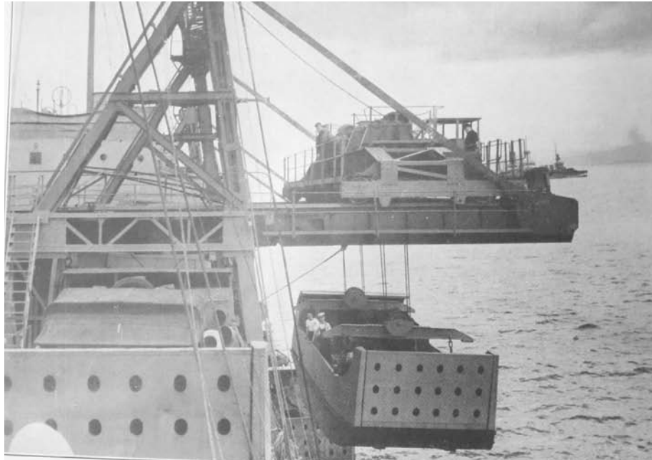
A LCM(Mk1), representing a self-propelled open-topped box, being lowered by a boom-supported transporter crane [author's collection]
